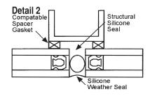
For insulating glass, the design must be changed to accommodate Figure 1 and Detail 2, unless a one component silicone secondary seal is used.
