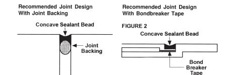
Lap-Shear Joints should have a bead which is equal to, or greater than, the total anticipated movement.
