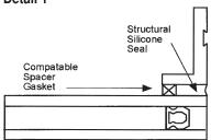
DETAIL #1 is commonly used in shop glazed applications where a glazing insert or split mullion is used. Care should be taken in applying the structural sealant to avoid direct contact with the insulating glass edge seal. The cure by-products are free to dissipate into the surrounding atmosphere and would not be entrapped in direct contact with the silicone I/G seal.
